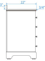
\*Note: Due to high probability of breakage, the backsplash comes in two pieces, cut from same piece. All measurements are  $\pm$  1/4".
